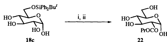
Scheme 8 Reagents and conditions: i, CCL, CH 2 Cl 2 , PrCO 2 CH 2 CCl 3 , 75%; ii, Bu 4 NF/AcOH, -50 °C, THF, 75%
